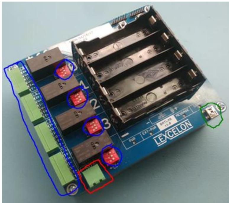
**BLUE:** These are external headers that may be used to connect the Batlab to a non-18650 cell slot tray. The red dip-switches must all be flipped to the off (downward) position to use the external headers instead of the 18650 form factor sized tray that is soldered to the Batlab.
